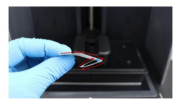
5.3.1 Using the menu on the printer touch screen, select the "Function" icon, "Z-axis Movement", then select the "Z 0" icon. The build plate will descend to the button and press down on the paper strips and leveling paper.
