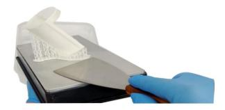
After removal, the model should be cleaned in minimum of 95% alcohol for several minutes, time depends on the model's complexity and size.
